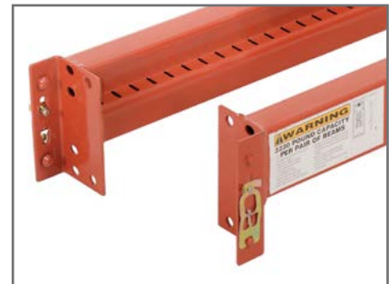
Heavy Duty Cross Shelf Beams: High strength 15 gauge steel beams have a 1-5/8" H step beam design that accommodates cross bars and decking.
