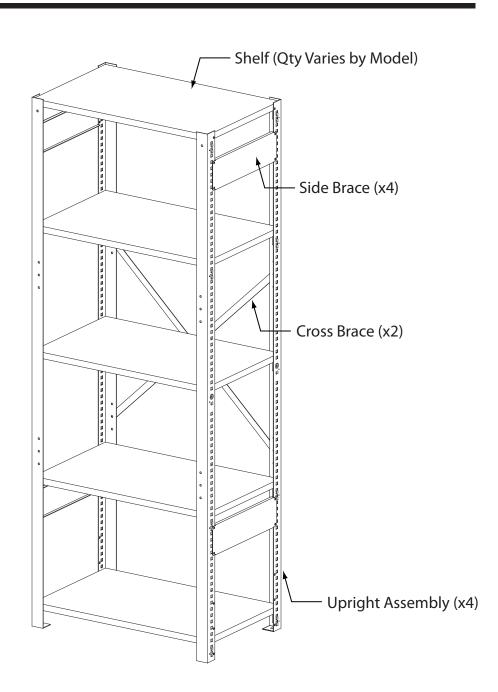
Assemble as illustrated. Lay two uprights out and attach two side braces between uprights using 4 bolts/nuts per side brace.
